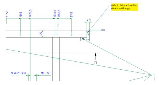
All non-tolerated dimensions and unmachined surfaces of welded parts shall be manufactured in accordance with the general tolerance DIN EN ISO 13920 B.
