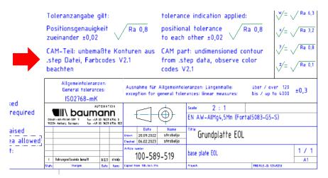
only elements that are not defined by contour or color of the 3D model are dimensioned:
