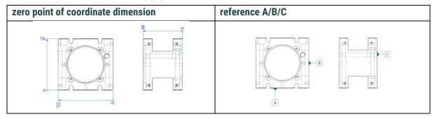
For undimensioned elements, the following always applies: The dimension from the zero point is assigned the corresponding tolerance (general tolerance or tolerance assigned via colour). Example: for the edge marked in green, dimension 60 applies with the corresponding general tolerance.
