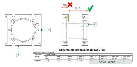
If the 3D model and the drawing contain contradictory information, the information on the 2D drawing shall apply.
