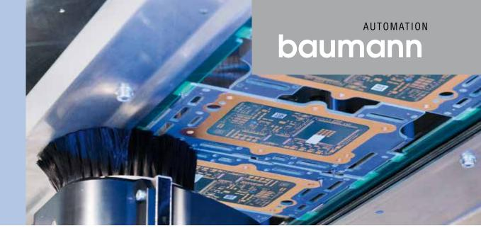
The tool is automatically checked for crack after each milling operation to ensure maximum process reliability. An automatic tool changer enables a number of tools to be stored in the magazine. Continuous displacement of the milling tool helps to extend its service life considerably. Tools are changed out according to individually configurable parameters. Milling contours are generated using data transferred from the CAD in combination with tool parameters.
